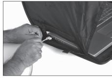
Similar openings on the left and right sides allow access to ports on either side of the laptop.
